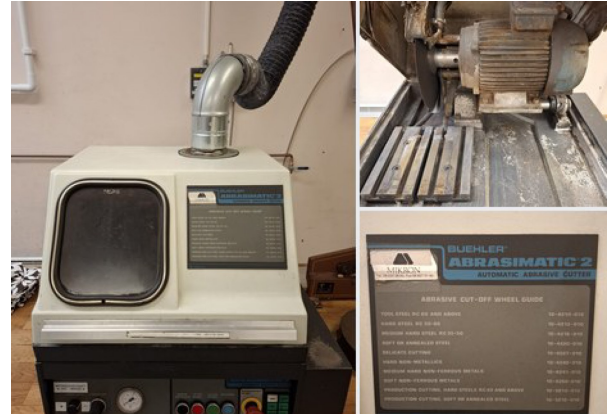
BUEHLER ABRASIMATIC 2 abrasive cutter, Erasteel Vikmanshyttan
