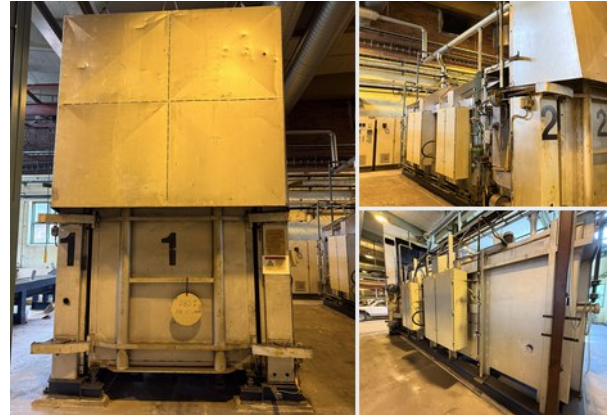
H 2 batch annealing furnaces (×2, sub-lots 18A & 18B), Erasteel Vikmanshyttan
