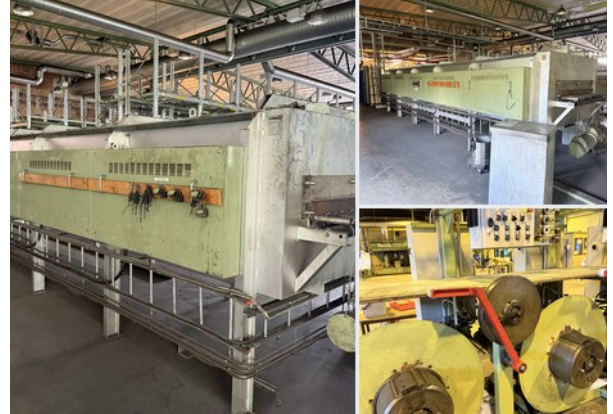
Ovens 5–6 narrow strip stretch annealing furnace (UTAB), Erasteel Vikmanshyttan
