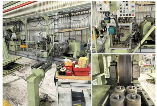
NDT / eddy current inspection line, Erasteel Vikmanshyttan
