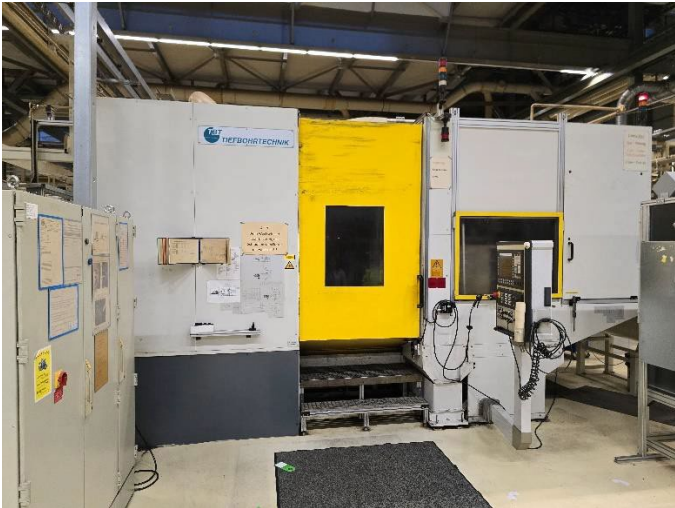
NILES N 30 MCM x 2.500 crankshaft turning, milling, turn-broaching and drilling machines
