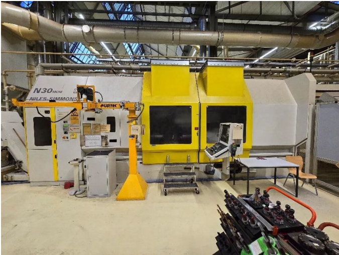
NILES N 30 MCM x 2.500 crankshaft turning, milling, turn-broaching and drilling machines
