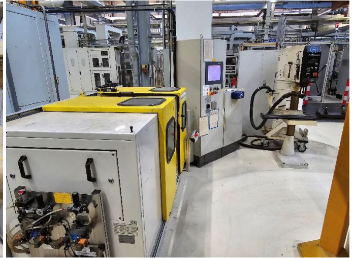
HEGENSCHEIDT 7794 bearing fine turning+finishing HEGENSCHEIDT 7893R deep rolling+straightening HOFFMANN pre-balancing (manual)
