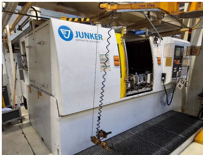
JUNKER JUNCRAK 6000/50-50 (2 of) and JUMAT 5000/60 crankshaft grinding machines
