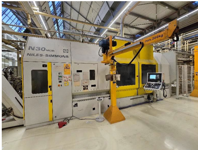
NILES N 30 MCM x 2.500 crankshaft turning, milling, turn-broaching and drilling machines
