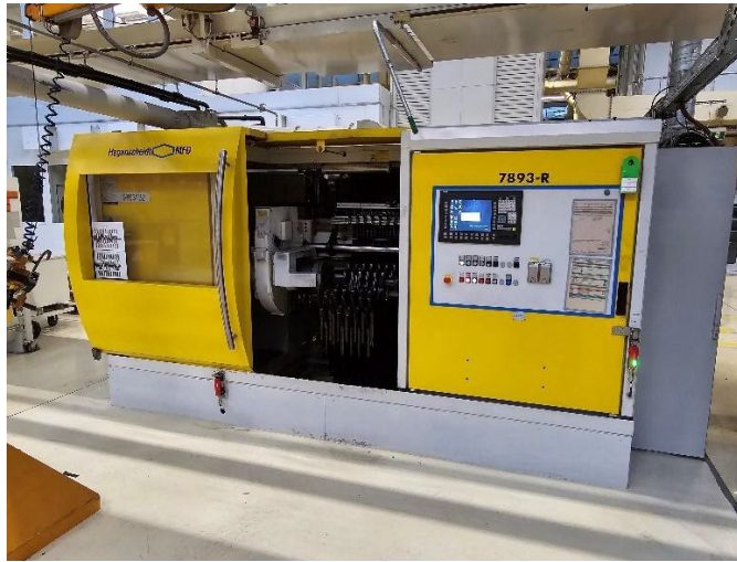
JUNKER JUNCRAK 6000/50-50 (2 of) and JUMAT 5000/60 crankshaft grinding machines
