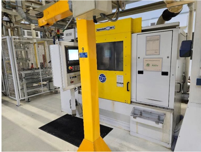
JUNKER JUNCRAK 6000/50-50 (2 of) and JUMAT 5000/60 crankshaft grinding machines
