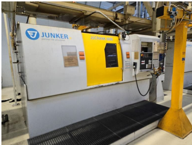
JUNKER JUNCRAK 6000/50-50 (2 of) and JUMAT 5000/60 crankshaft grinding machines
