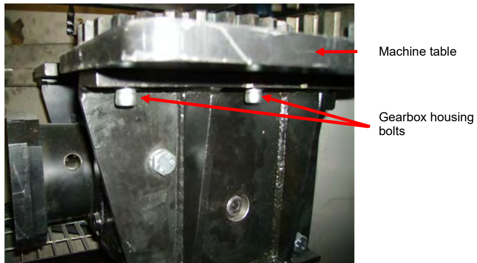
Figure 15 : Gearbox Housing Bolts
