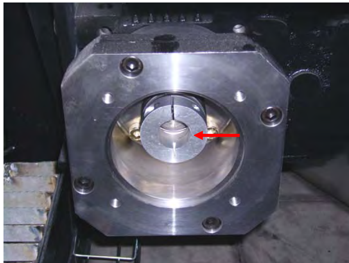
Figure 7 : Motor Coupling (with motor removed)
