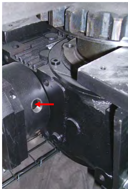
Figure 5 : Gearbox Access Aperture
