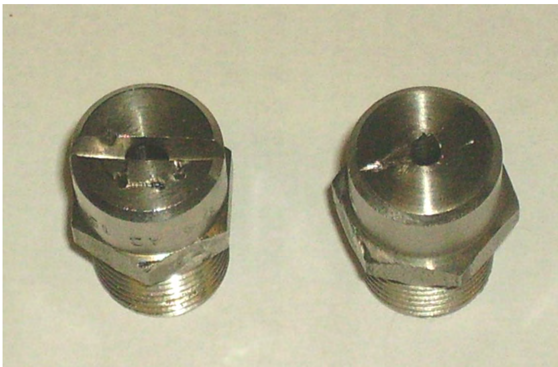
Figure 25 : Typical Wash Jet Damage
