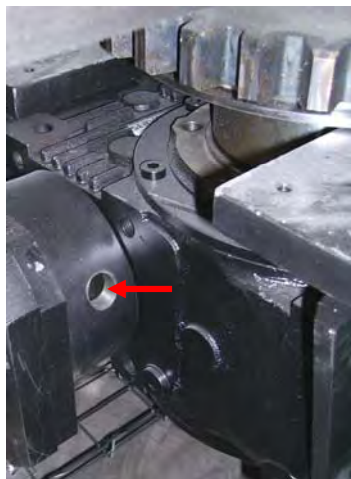
Figure 10 : Gearbox Access Aperture
