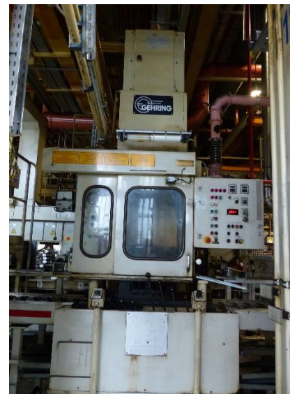
GEHRING Z-350-125 (1992) – Manual Vertical Honing Machine
